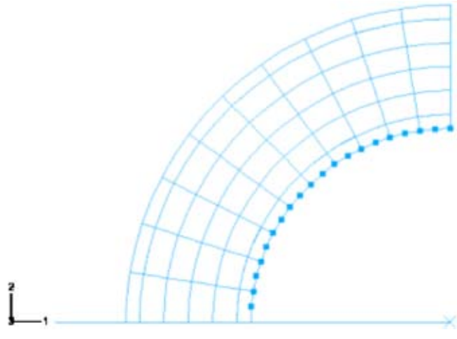
Fig. 9 Typical finite element mesh used in the correlation analyses
