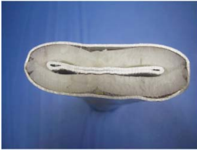
Fig. 8 Collapsed cross section of specimen PIP.M2.G1.I02
